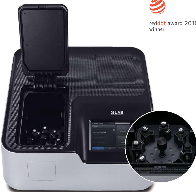
The previous single beam type spectrophotometer has a weak point of error occurrence in measuring a sample, because of the movement of a light source by time lag in measuring the strength of between a reference light and a light from sample. To solve the problem, OPTIZEN Alpha was designed as a double-beam type spectrophotometer. The system utilizes an additional reference beam to improve the measurement performance by compensating the intensity fluctuation of its light source.
