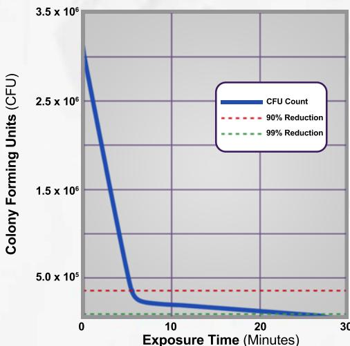
Adjustable pipettes were inoculated with S. aureus and placed in the UV Pipette Carousel. Individual pipettes were removed during the Auto-Decon™ cycle at various intervals and rinsed to collect any residual contamination. The rinses were then plated and the CFU counted to determine the effectiveness of a single decontamination cycle.
