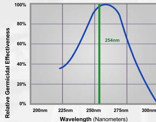
The blue curve, above, shows the germicidal effectiveness of UV light on E. Coli. The green line represents the 254nm wavelength of industry standard germicidal lamps like the one at the core of the nUVaClean's pipette chamber. This lamp emits greater than 90% of its light at 254nm, which causes damage to the DNA of microorganisms, preventing their growth and reproduction, ultimately destroying them (see Figure 1.).
